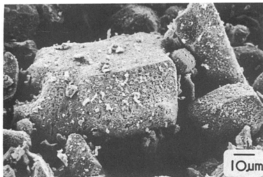
Figure 11 Scanning electron micrograph of product of reduction of "Cerac" cobalt tungstate at 700° C.
