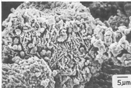
Figure 13 Scanning electron micrograph of product of reduction of "Cerac" cobalt tungstate at 1100° C.
